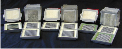
Fig. 3. Open calorimeter blocks. The long bottom calorimeters have two-sided, the side calorimeter one-sided readout
